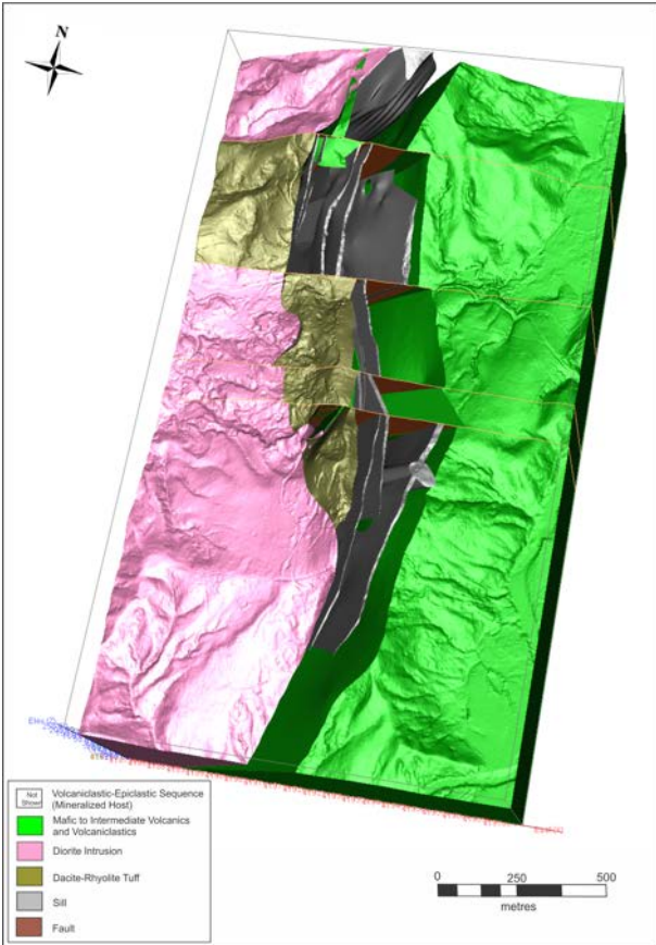
Figure 1: Plan view of Alacran geological model showing generally west-dipping lithostratigraphy, with mafic to intermediate volcanics & volcanoclastics in the east and footwall to the main copper-gold mineralised zones hosted mainly by volcanoclastic -epiclastic sequence that is intruded by intermediate sills and also larger dioritic bodies in the west and north. Mineralization also locally overprints the intrusions.
