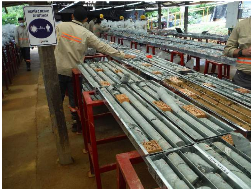
Figure 12.7 – Core Logging Facility at the El Alacrán Camp
