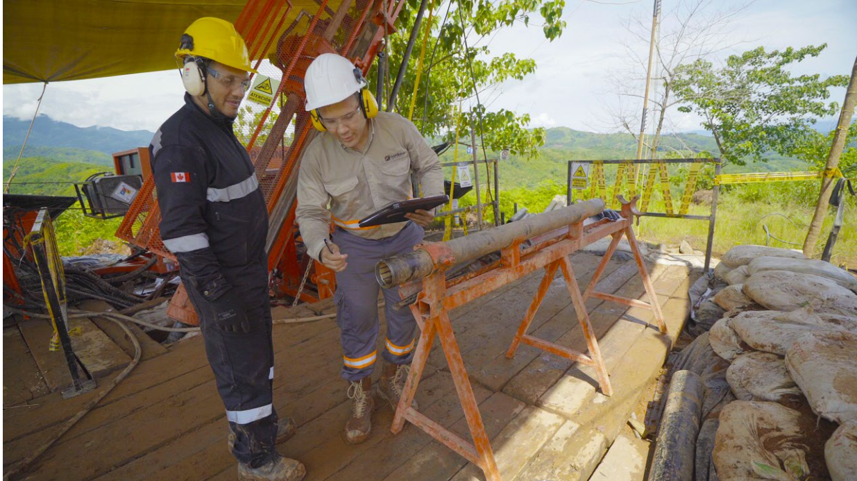
Jaime Aroca, Chief Geologist, with Anibal Quintero, a member of the drilling team to inspect the core barrel and monitor the quality of the core samples at the Alacran Project.
